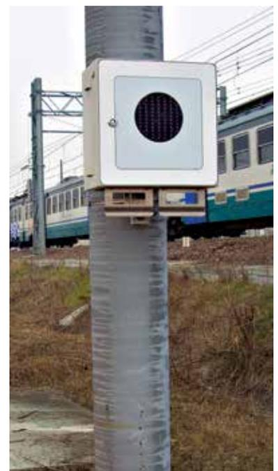
projects, such as bridge renewals or tunnel upgrading works, the ATWS can be installed on a long-term basis with the equipment connected by cable. However, these can take a long time to complete, so a portable version using radio links has been developed for short-term applications.
