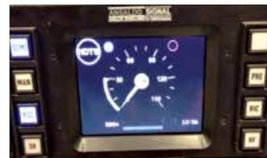
Fig 1. HDTS uses coded track circuits overlaid on the conventional signalling to shorten block sections and increase capacity on busy lines.
